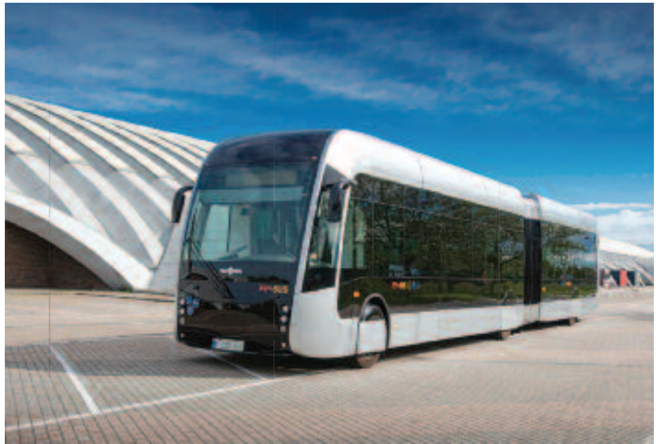
At the cutting edge of technology is the Keolis operation in Pau, France. It includes a six-kilometer Bus Rapid Transit (BRT) line serving 14 stations. The buses are 18-meter articulated tram buses using hydrogen-electric power systems. VAN HOOL.
