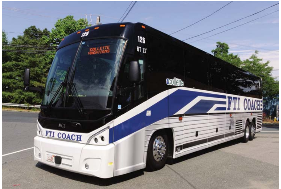
The most interesting new addition to the FTI Coach fleet carries fleet number 126. Although a new MCI J4500, the "silversiding" was added to give it a retro look. Although not obvious in this photo, the stainless steel siding appearance was created by an MCI external wrap.
