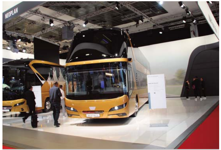
Originally introduced in 1967, the double-deck Neoplan Skyliner model has been in production for 52 years. This one had steps going up on the right side and a kitchenette on the lower deck. Note the new Opti-view cameras instead of mirrors.
