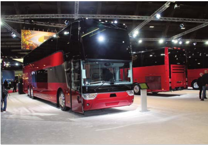
Van Hool had eight buses on display with six of them being coaches painted red. The TX 27 double-deck Astromega had a ZF Traxon transmission and a seating capacity of 89 plus driver and tour escort. Nearby, an EX15 model had right-hand drive for the British market.
