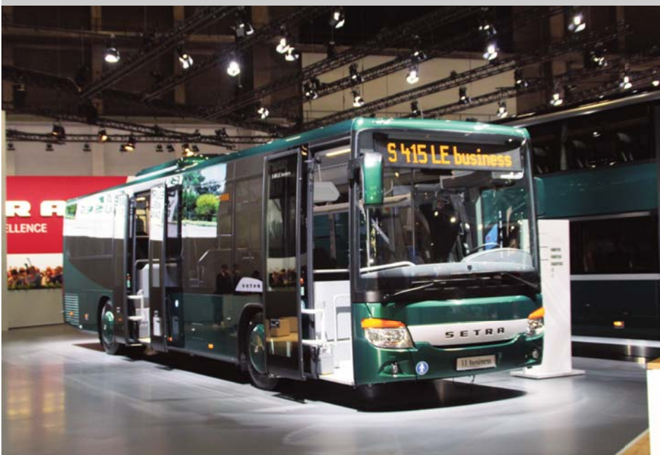
Setra had four coaches in display and offers three different classes. This is their S 415 LE Business model that belongs to their ComfortClass. It is effectively a two-door, low-entry suburban and can accommodate mobility devices with a ramp at the center door.
