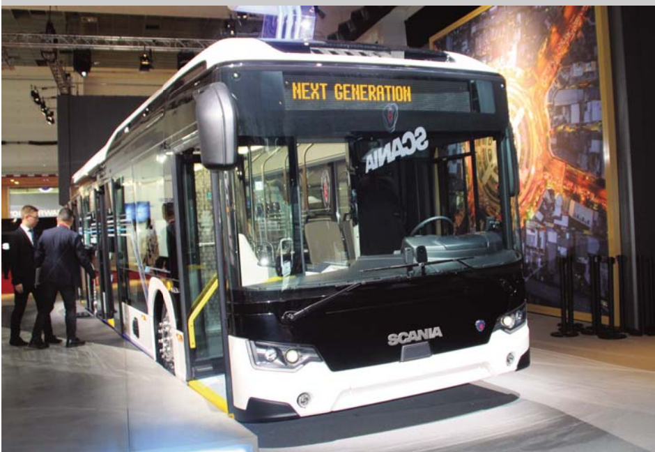
Scania unveiled the battery-electric version of their Citywide transit bus. It is 12 meters long, had three doors and has a range of 80-150 kilometers. Scania has been part of the Volkswagen organization for several years but retains its traditional name.
