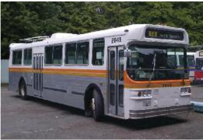
Bus 2649 is a Flyer E800 originally built as a trolley bus in 1976. Similar buses in the fleet were dieselized in the 1980s but 2649 retained its trolley poles for use as a trolley wire deicer. It was recently restored by the TRAMS volunteers.
