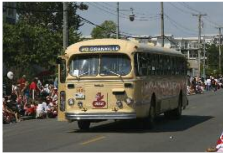
Bus 3405 is a 1957 Canadian-built CCF Brill CD52A. It originally operated for BC Electric and is painted in the original livery it had when delivered. The TRAMS collection also includes two Brill trolley buses and a similar diesel bus.
