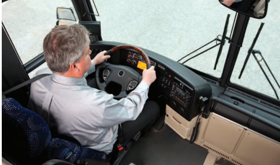
The Prevost PRIME system monitors battery charge, air pressure and engine torque without any intervention on the part of your driver. It makes the appropriate decisions to maximize fuel efficiency and minimize pollution. However, a new gauge has been added to the dash to let the driver know when the coach is running on "free electricity."
