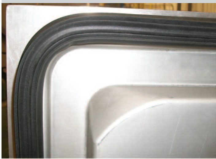
Although twice as thick as previous doors, the aluminum luggage bay doors will reduce weight by 265 pounds per coach.
