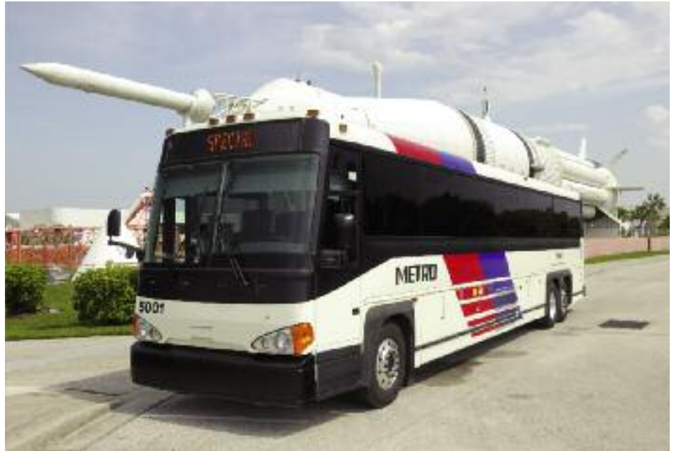
MCI pioneered hybrid Commuter Coaches in 2003 with coaches for New Jersey Transit. Houston Metro placed a major order for MCI hybrid Commuter Coaches in 2007. Shown here, the Houston hybrids are 45 feet long with the Allison hybrid system and a Cummins engine.
