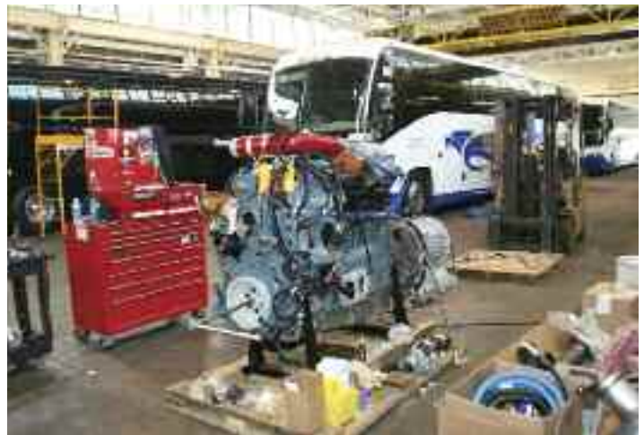
For repowers that must comply with EPA 2003 regulations, MCI uses rebuilt Detroit Diesel series 60 engines. This one already has an Allison transmission.
