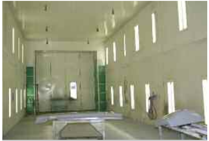
Loudonville has its own professional paint booth with the equipment to bake on the new paint. Painting is important in collision repair, refurbishing and pre-owned coach work.
