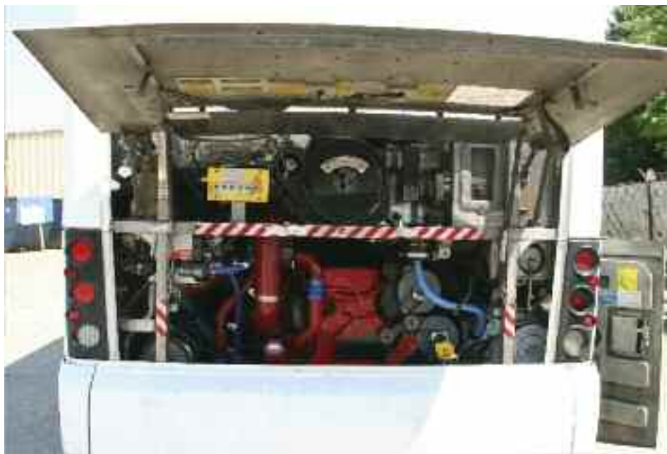
This pre-owned coach was sent to Loudonville for an engine repower. Complying with EPA 2007 regulations, it was repowered with a new Cummins ISM engine. This procedure has been so well regarded that customers are purchasing the coaches sight unseen even before Loudonville completes them.
