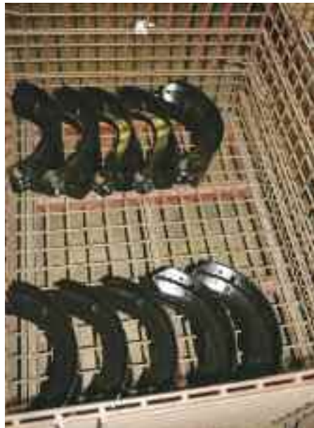
Loudonville has become MCI's center for brake shoes. Take offs and used brake shoes are disassembled and rebuilt. Loudonville also puts together new brake shoe assemblies.
