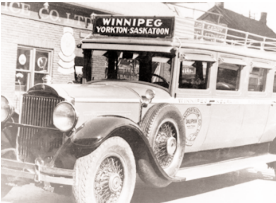
The Fort Garry Motor Body and Paint Works delivered its first bus in 1933. Built on a Packard chassis, it offered seating for 11 passengers and was operated on a route from Winnipeg to Saskatoon. MCI.
