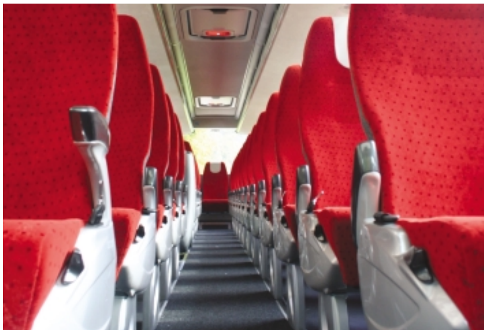
An additional concern for both seats and seat belts is sufficient anchoring. Anchoring seat belts to the floor limits the ability to respac seats if needed. When seat belts are incorporated into the seats, the seats will require additional anchoring because of the added stress. Shown here is the interior of a European Jonckheere bus. VDL.
