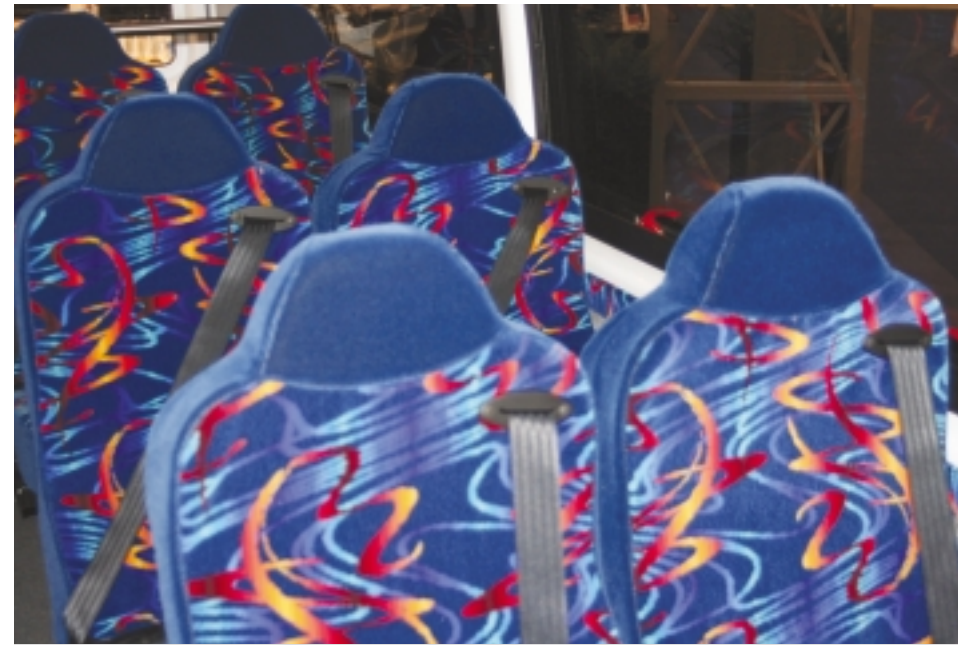
Seat belts are becoming increasingly popular on American buses. This 2006 photo shows a Sprinter with built-in three-point seat belts. Many large coaches are now also offering seat belts. NBT.
