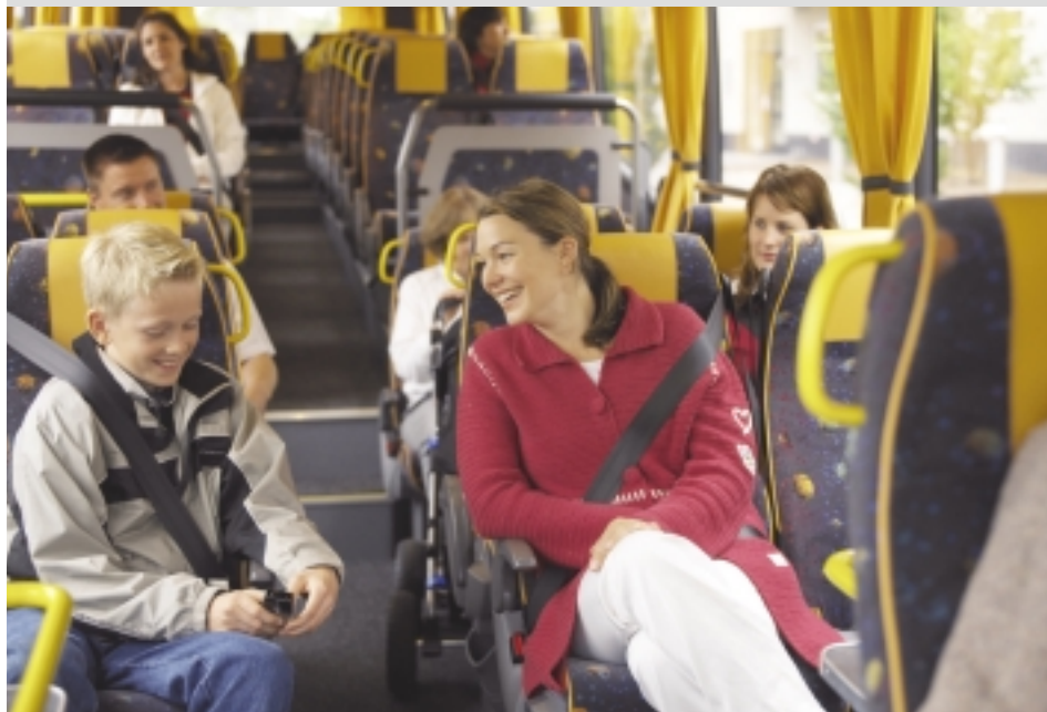
Europeans are more likely to take public transportation and more likely to use seat belts. Shown here is a Volvo 8700 bus with three-point seat belts. Three-point belts are now available on some American coaches. VOLVO.
