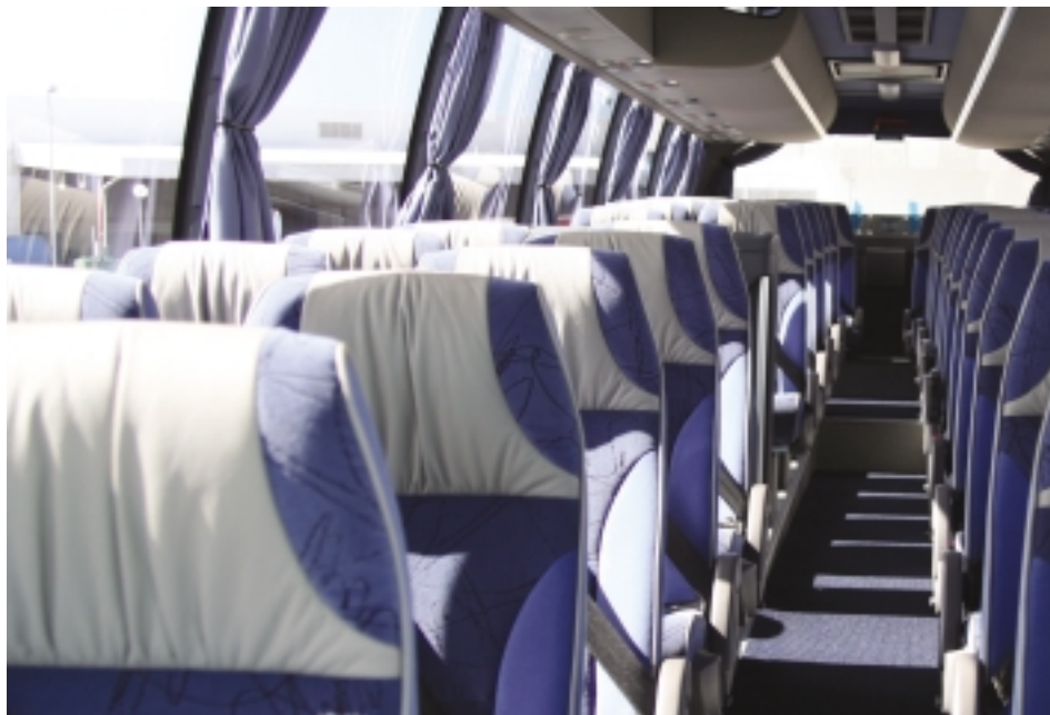
Push-out passenger windows are typically American. European buses have solid windows with little hammers to break the glass in the event of an emergency. Here is a European Volvo 9700 with three-point seat belts and European solid passenger windows. VOLVO.
