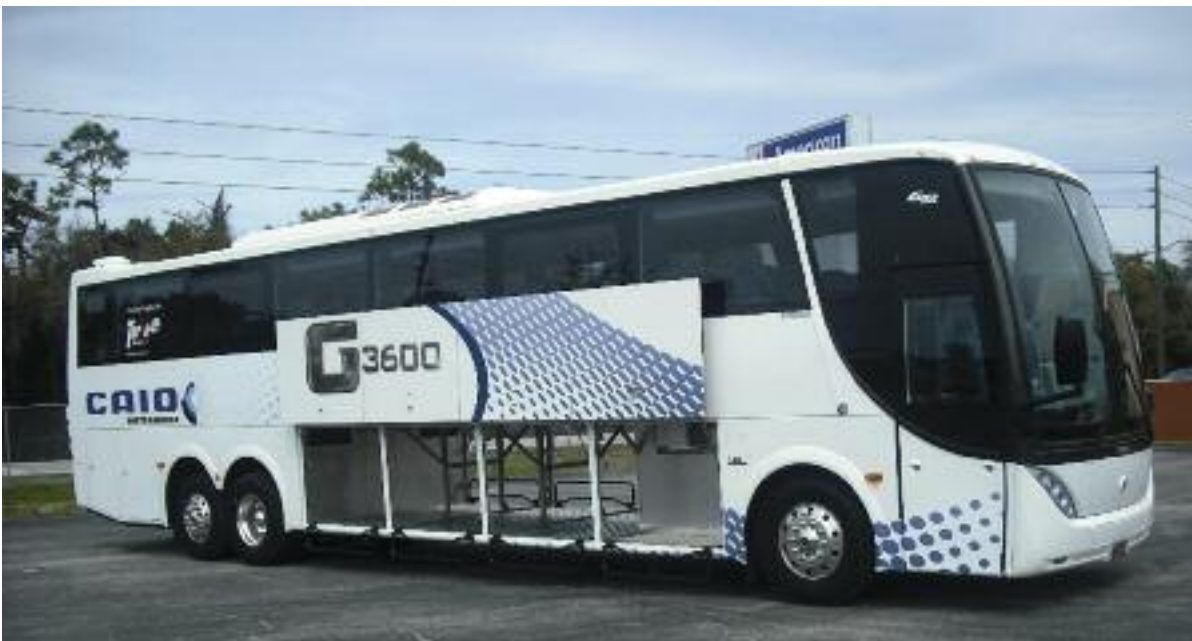
The CAIO G3600 is a full-size, 45-foot motorcoach that offers 477 cubic feet of luggage area.
