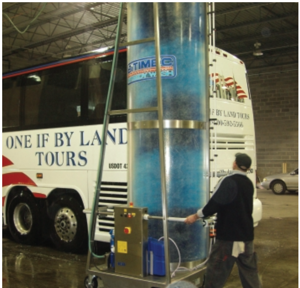
The 101 is the basic Speedy Wash model and does require both electrical and water connections. This unit is being used in a bus garage in Flushing, New York. The connections are overhead.
