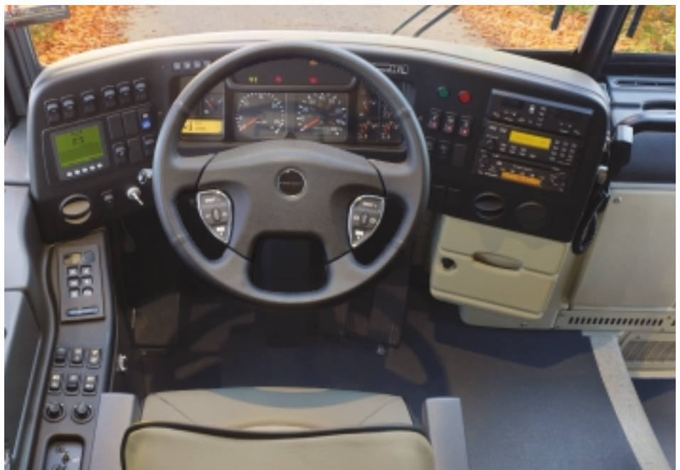
This photo shows the Beru Tire Monitoring System display mounted on this Prevost bus dash on the left side of the steering wheel. In normal operation, the driver can see the condition of all tires at one glance. In the event of either a pressure or temperature problem, the system will notify the driver.
