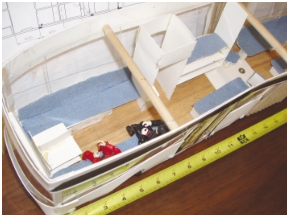
This photo shows the back end of the Lightrider articulated bus model. At the top right is a driver's bunk located atop luggage shelves. The square structure immediately behind this is the restroom. Between the two couches at the rear is a shelf designed to carry six duffel bags. LIGHTRIDER MINISTRIES.
