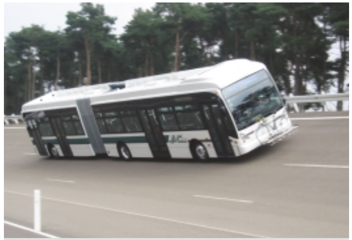
The Van Hool AG300 articulated buses order by AC Transit were put through a series of tests. Here, one of the articulateds is tested performance at higher speeds. The AG300 is a tractor-trailer with an under-floor engine in the front unit. ABC COMPANIES.
