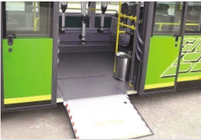
One of the obvious advantages of the low-floor bus is the ease of entry and exit. With so many bus passengers being elderly, a low-floor entrance door has obvious advantages. This photo shows how easy it is to deploy a ramp from a low-floor door for wheelchairs and other handicapped vehicles. DAIMLERCHRYSLER.
