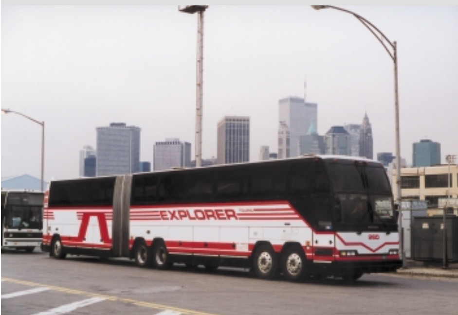
This Prevost H5-60 articulated coach was photographed in Brooklyn in 1995. This model has operated successfully for two decades but is more like a conventional coach because of its high-deck design. It has both a front and a rear door. J.C. REBIS JR.
