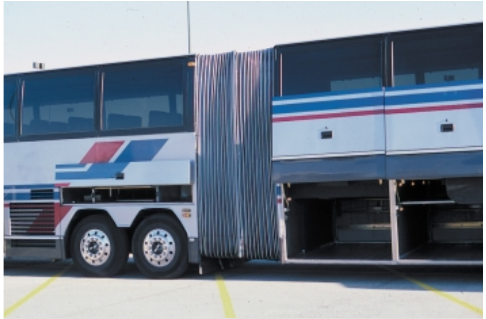
The Prevost H5-60 offers underfloor luggage space and a higher deck for better passenger viewing. While a low-floor bus would provide easier entry and exit for passengers, the passengers' view would not be as nice and dealing with the luggage might present problems. NBT PHOTO BY LARRY PLACHNO.
