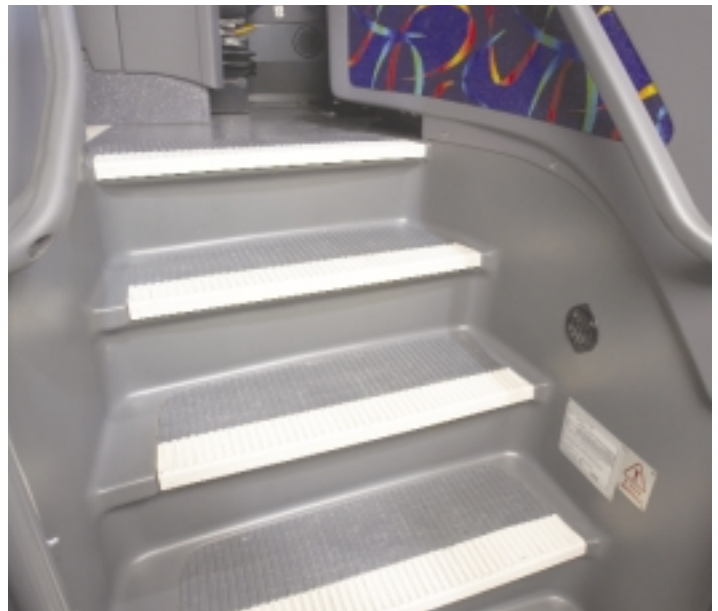
The front stepwell has been completely redesigned. Safety is improved with white nosed rubber step treads and a nice handrail to assist passengers while boarding.
