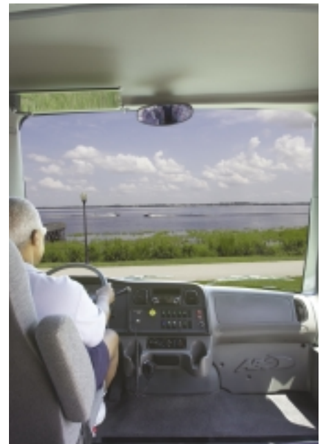
The new one-piece windshield improves safety by giving the driver an unobstructed view to the front. It also improves viewing for the passengers.
