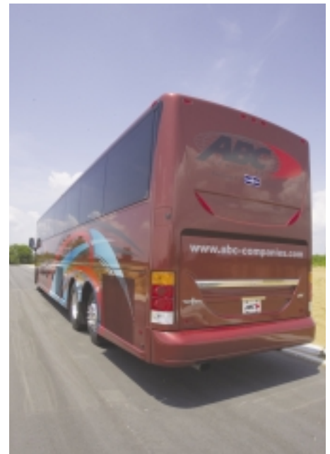
The rear of the coach has been redesigned with a new cap, more rounded body lines and LED lighting although the pantograph engine compartment door remains.
