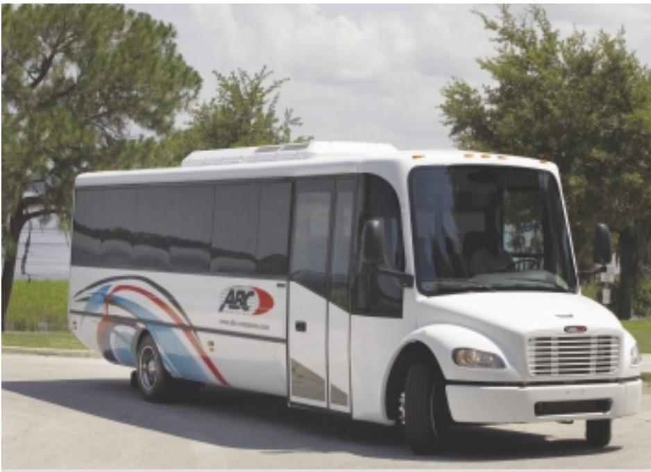
One of the major improvements on the new M1235 is an improved chassis with increased wheelbase. The new front design, which includes a one-piece windshield and new hood is obvious. Noteworthy also is the upgraded interior with fiberglass trim panels.
