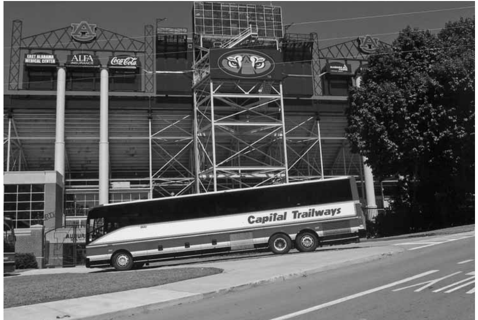
Coach 99367 was recently photographed while on a charter. It is a 45-foot, 57-passenger Van Hool C2045 built in 2005. Today's latest paint scheme is traditional Trailways red and white with the addition of a blue stripe and the company name in blue.
