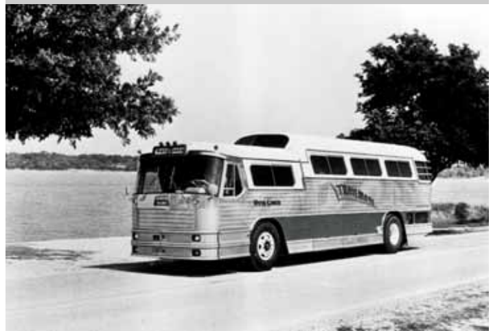
Trailways carriers operated a wide range of different coaches. Flxible Clippers and later Flxible models such as this VL-100 were popular on lighter routes, particularly in the years after the War and before the new Eagles became popular. NBT COLLECTION.
