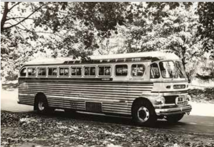
The ACF-Brill buses were powered by an underfloor Hall-Scott gasoline engine and were popular with several Trailways companies. This one was operated by Safeway Trailways, one of the original five Trailways founding companies. NBT COLLECTION.
