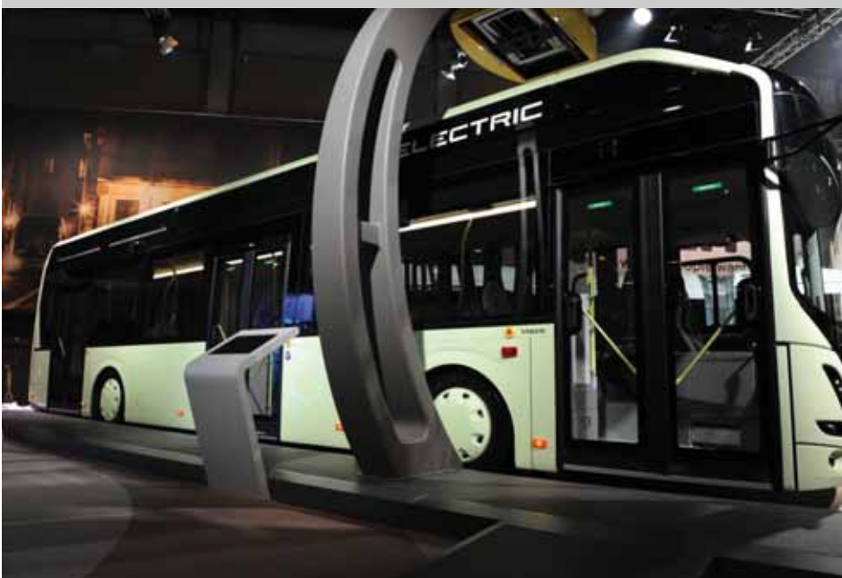
Busworld saw the debut of the new all-electric 7900 transit bus from Volvo. It has a length of about 39.3 feet and operates totally on battery power. It is interesting that a major engine builder like Volvo is keeping up with the trend to electric transit buses. BUSWORLD.
