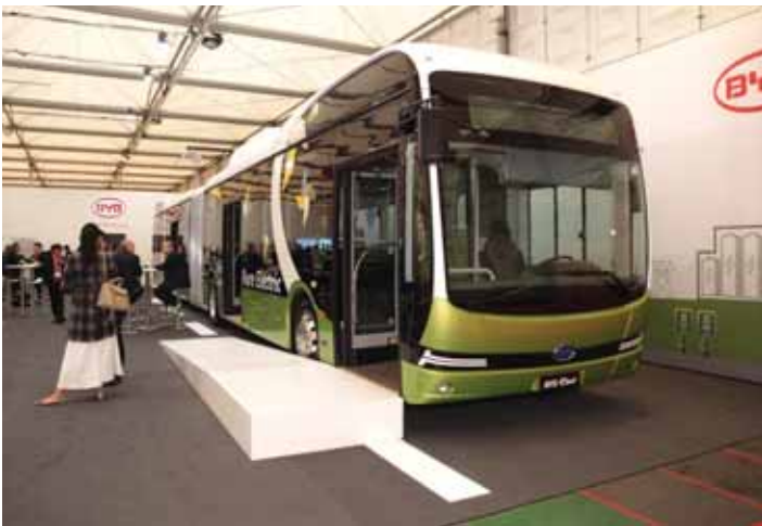
BYD showed their new 18-meter (59-foot) articulated transit coach that was powered by batteries. It had a capacity of 150 passengers. OREN KIPNIS.
