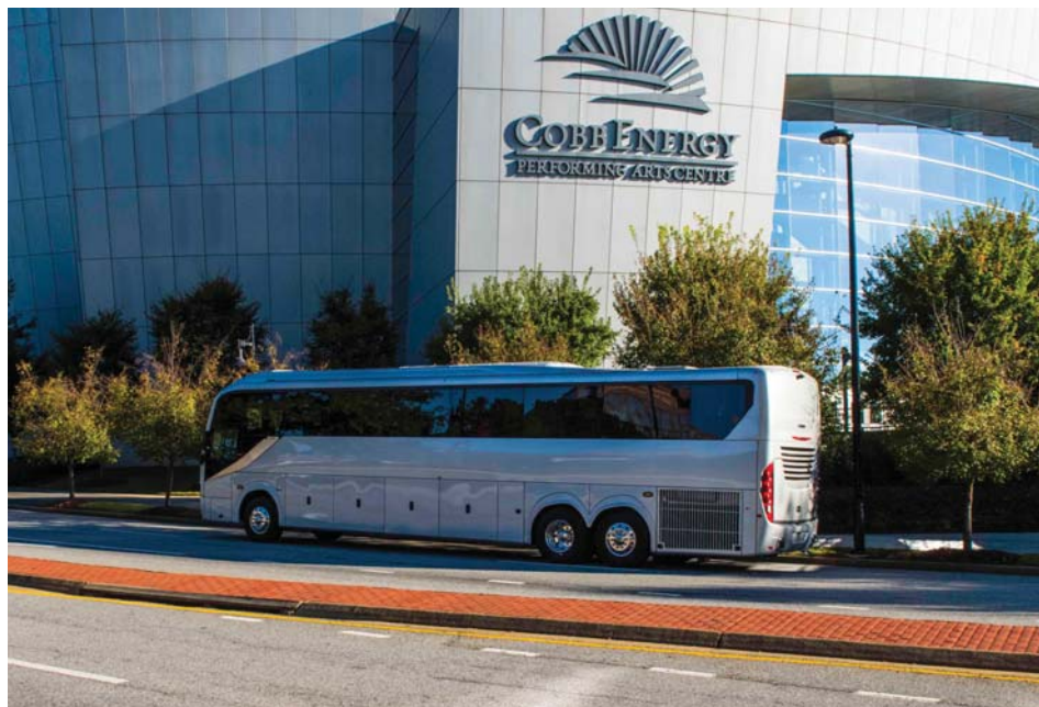
The new stainless steel CAIO models offer several improvements over the previous models. Noteworthy is the full exterior light package that uses longer-lasting LED lights. The American-made passenger windows are not glued in but are quick-change.
