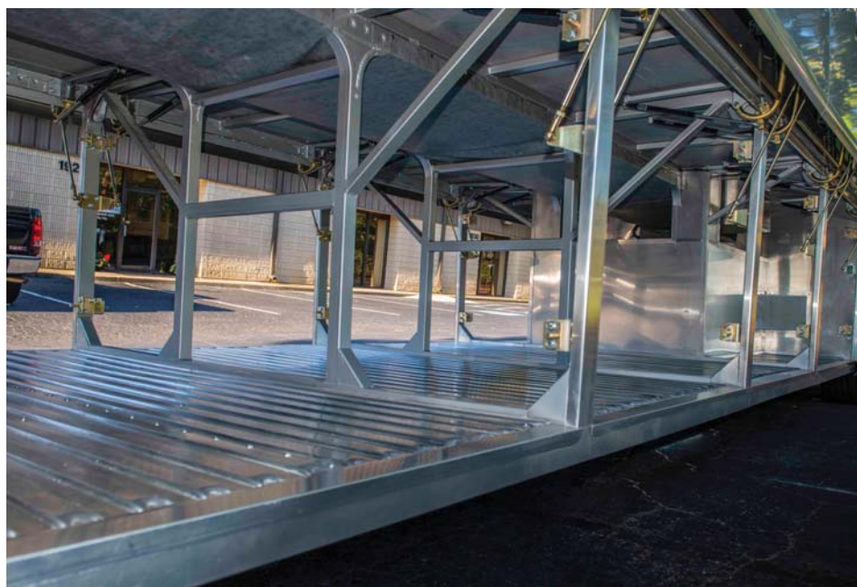
A major feature of the new CAIO S3645 is its huge underfloor luggage compartment. This 517 cubic feet of underfloor luggage space comes in very handy on longer charters and tours. A reduction in fasteners in the luggage compartment makes it easier to clean and reduces the potential for luggage damage.
