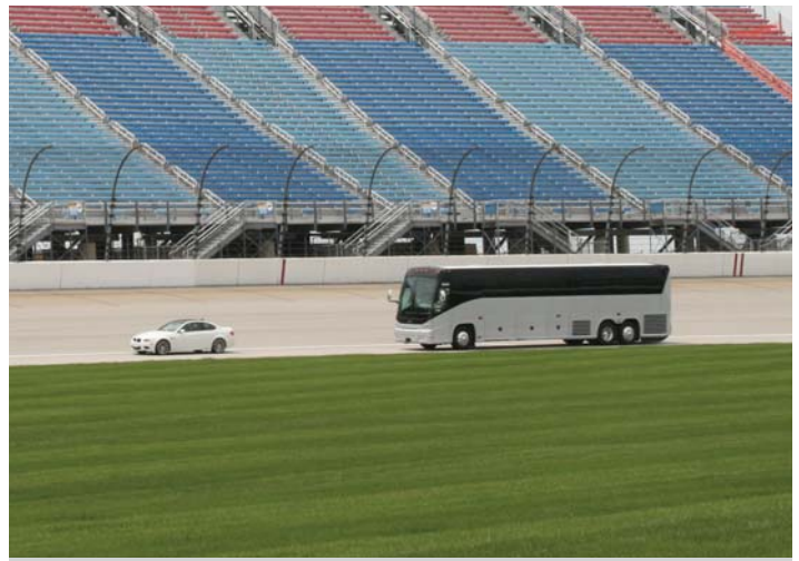
A car driven by Brent Maitland slowed down in front of the J4500. It was detected by the Wingman radar on the front bumper of the coach. First, it reduced throttle, then applied the Jake brake and finally applied the foundation brakes to maintain a safe distance.
