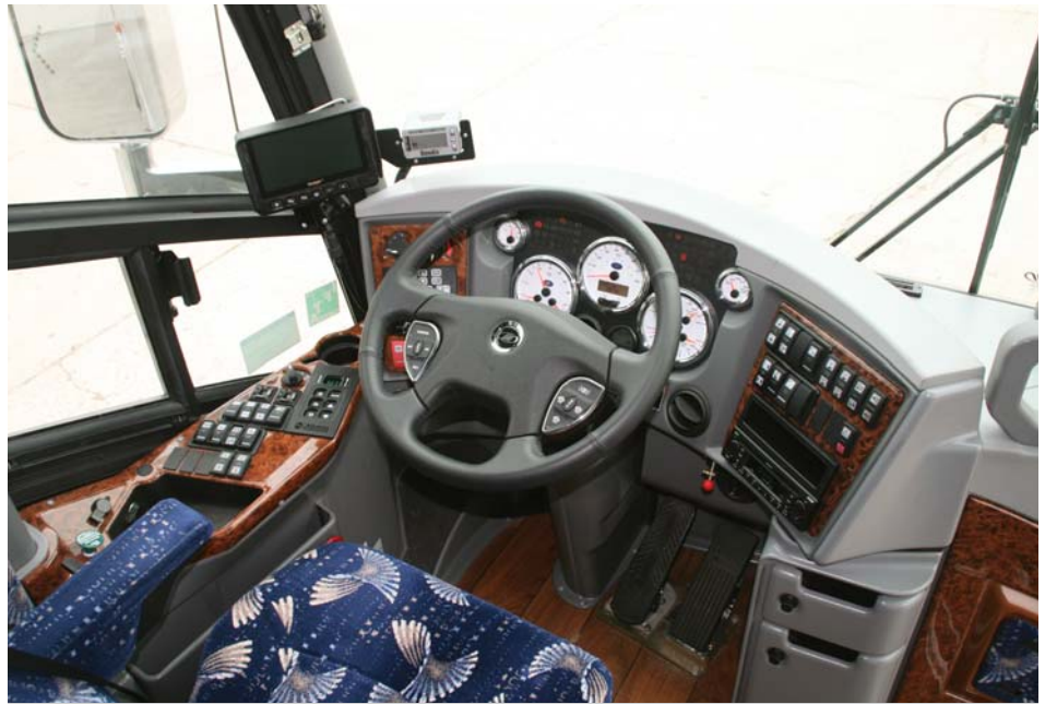
The driver cockpit area on the J4500 continues to be practical and very workable. I particularly liked the convenient controls on the smart steering wheel and the convenient left side panel with the transmission buttons. The new Bendix Wingman display is the small white box to the right of the center post. NBT.
