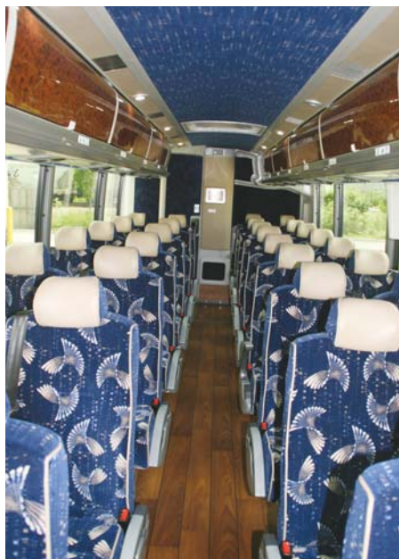
Other improvements worthy of note are the new parcel racks that hang down less and make the aisle more open as well as new passenger comfort modules under the parcel racks. NBT.
