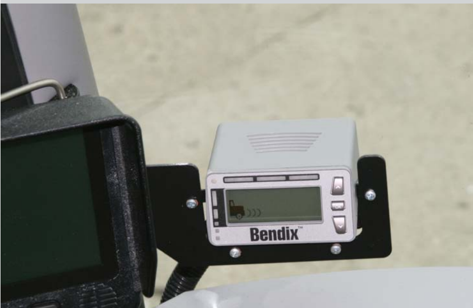
Here is a closer look at the Bendix Wingman display. While using cruise control, the Wingman system maintains a safe distance from the vehicle ahead by reducing the throttle, applying the Jake brake and then applying the foundation brakes if necessary. With cruise control off, it still alerted the driver to conditions ahead. NBT.
