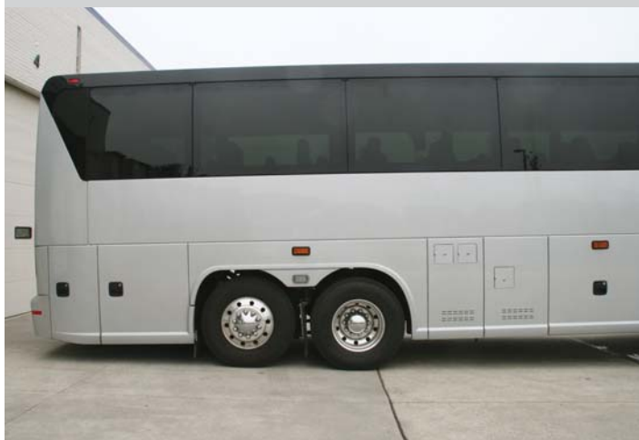
A ZF A 132 is now used as the drive axle on the J4500 while a ZF RL 80 E independent tag with a trailing or casting feature is used on the tag axle. NBT.
